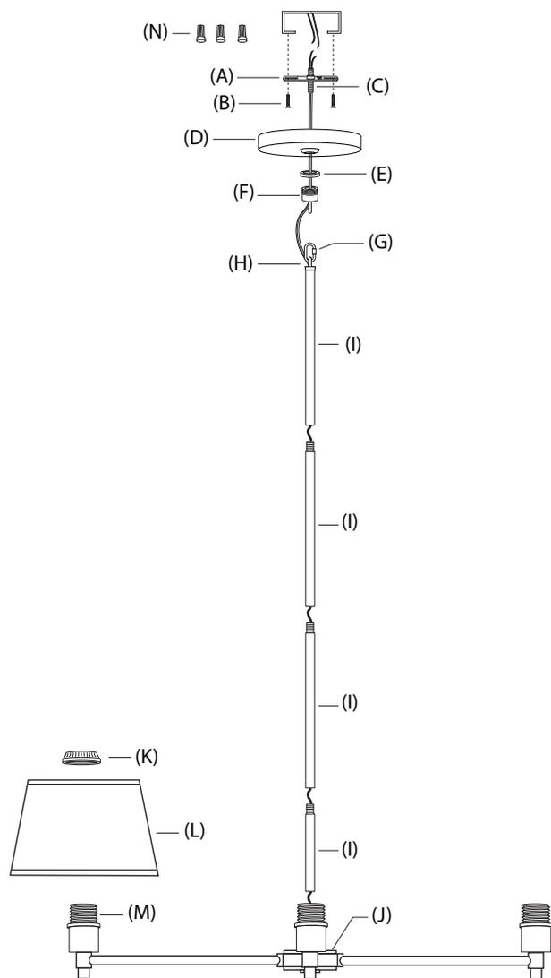
6. Measure desired drop for fixture to hang and add/remove extension tubes (I). Guide wiring through extension tubes before threading tubes together.
